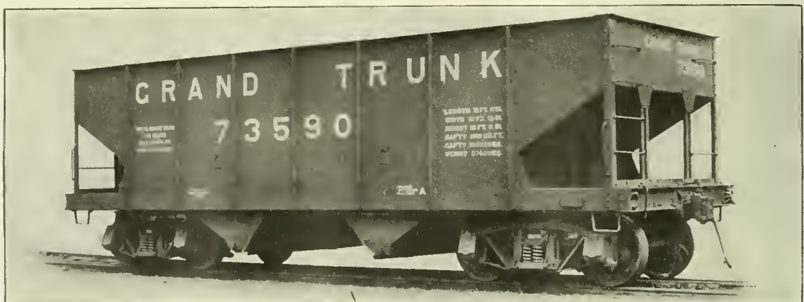
GRAND TRUNK 50-TON HIGH SIDE HOPPER BOTTOM STEEL GONDOLA.
